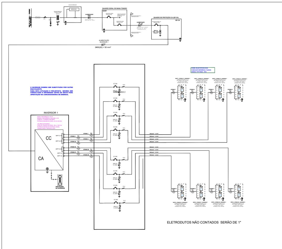
DIAGRAMA UNIFILAR SEM ESCALA
